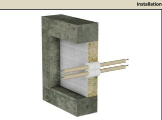
Electric conduit must be cleaned for dust. Debris and dust in the opening must be removed.
