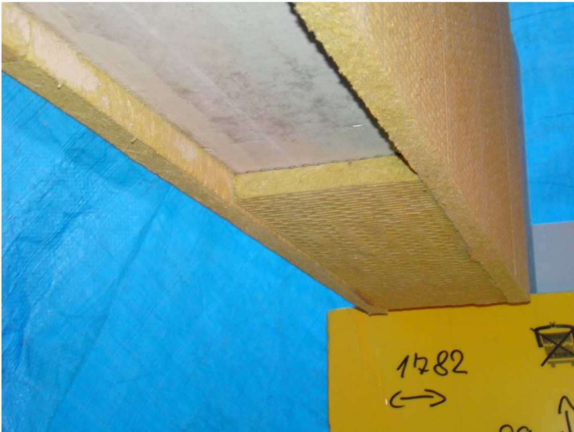
The flange is glued in the end.
